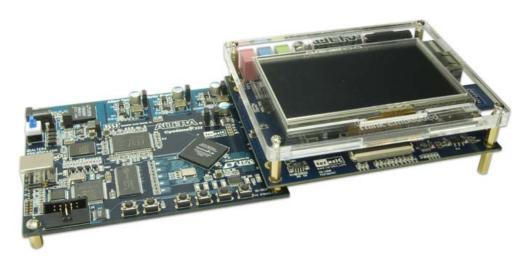
Figure 2. Connection of a MTDB Board and a Cyclone III Starter Board.
