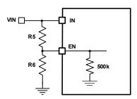
Figure 5: Adjustable UVLO using EN divider
