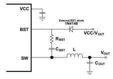
Figure 6: Optional External Bootstrap Diode to Enhance Efficiency
