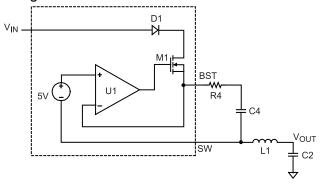
Figure 3: Internal Bootstrap Charging Circuit
