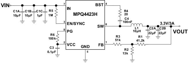
Figure 8: 3.3V Output Typical Application Circuit
