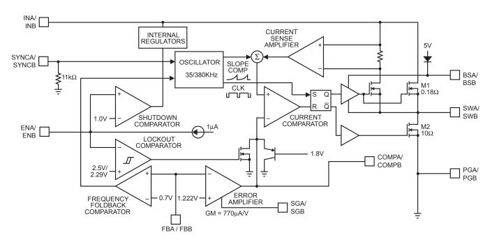
Figure 1—Functional Block Diagram (Diagram portrays ½ of the MP2362)
