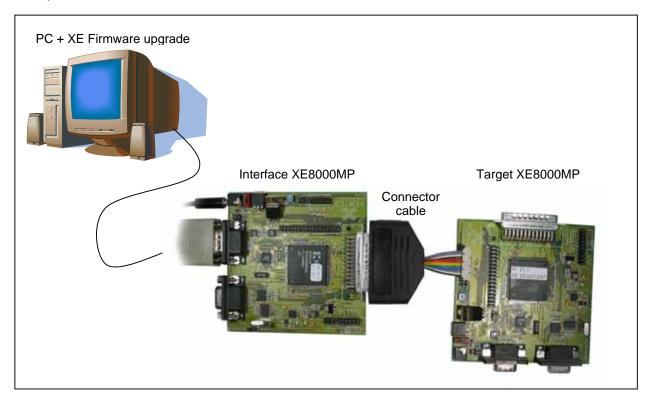
The zip file containing the new firmware also contains all the software necessary to do the upgrade. This means that you don't need to have RIDE installed, the XELoader and all the necessary drivers (.dll) are included in the .zip file. The only thing you'll need to do is to connect the XE8000MP's as shown above, power the Interface XE8000MP, connect it to the COM1 port (default) of the PC and launch the "upgrade.bat" file.
