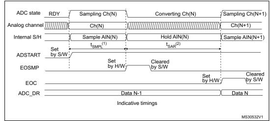
Figure 31. Analog to digital conversion time
