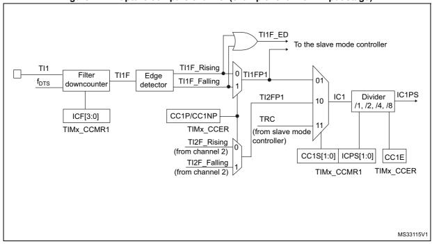
Figure 174. Capture/compare channel (example: channel 1 input stage)
