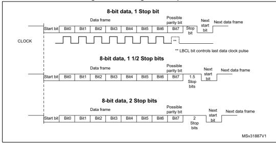
Figure 276. Configurable stop bits
