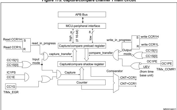
Figure 175. Capture/compare channel 1 main circuit
