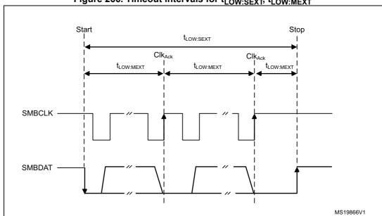
Figure 266. Timeout intervals for t<sub>LOW:SEXT</sub>, t<sub>LOW:MEXT</sub>
