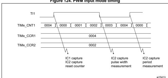
Figure 124. PWM input mode timing
