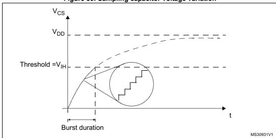
Figure 89. Sampling capacitor voltage variation
