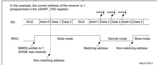
Figure 282. Mute mode using address mark detection
