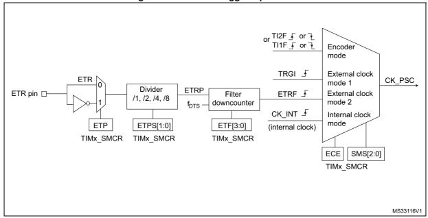
Figure 172. External trigger input block
