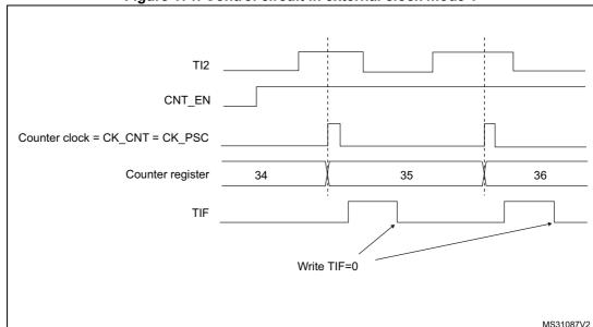
Figure 171. Control circuit in external clock mode 1
