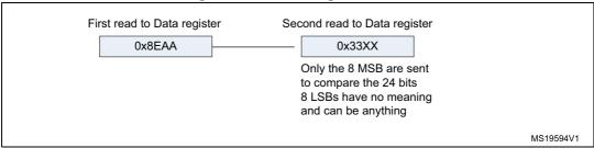
Figure 321. I<sup>2</sup>S Philips standard (16-bit extended to 32-bit packet frame)
