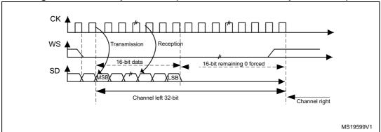
When 16-bit data frame extended to 32-bit channel frame is selected during the I<sup>2</sup>S configuration phase, only one access to the SPIx\_DR register is required. The 16 remaining bits are forced by hardware to 0x0000 to extend the data to 32-bit format.
