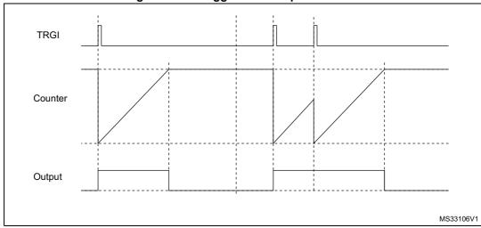
Figure 185Retriggerable one pulse mode
