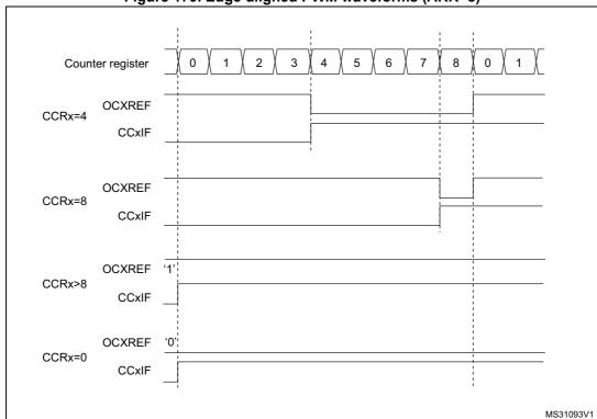
Figure 179. Edge-aligned PWM waveforms (ARR=8)
