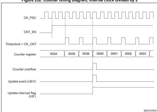
Figure 232. Counter timing diagram, internal clock divided by 2
