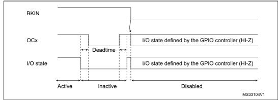
Figure 136. PWM output state following BKIN assertion (OSSI=0)
