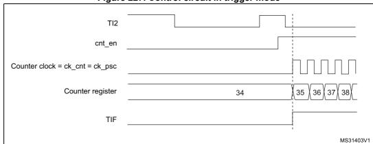
Figure 227. Control circuit in trigger mode
