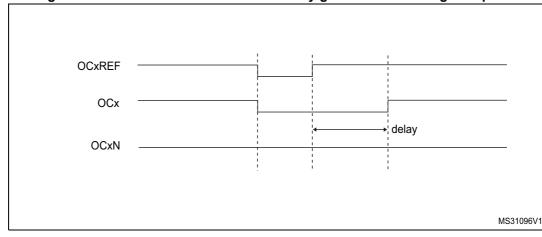
Figure 220. Dead-time waveforms with delay greater than the negative pulse.
