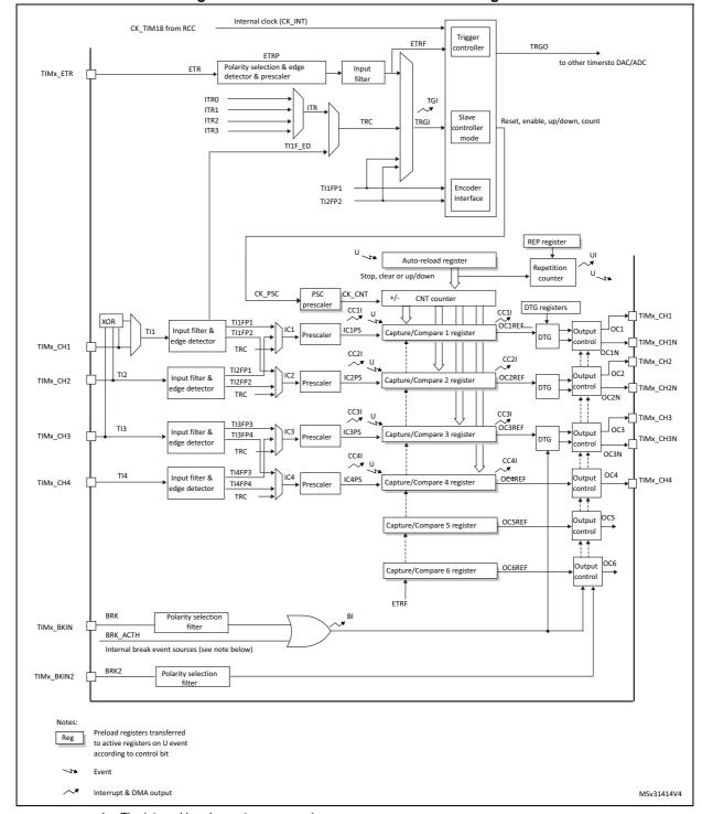
Figure 92. Advanced-control timer block diagram
