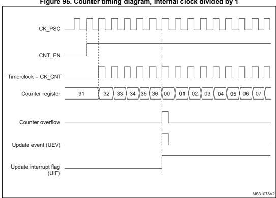
Figure 95. Counter timing diagram, internal clock divided by 1
