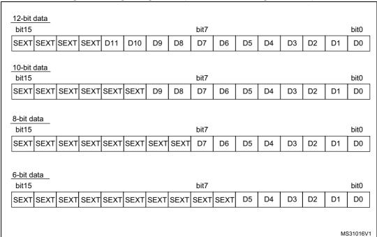
Figure 55. Left alignment (offset disabled, unsigned value)
