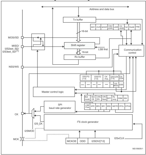
1. I2S2ext\_SD and I2S3ext\_SD are the extended SD pins that control the I2S full duplex mode.
