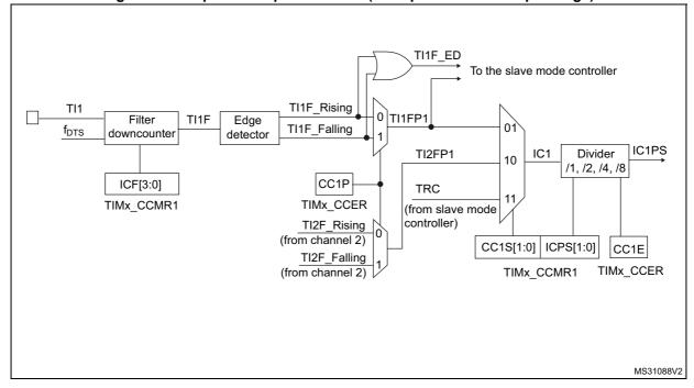
Figure 211. Capture/compare channel (example: channel 1 input stage)
