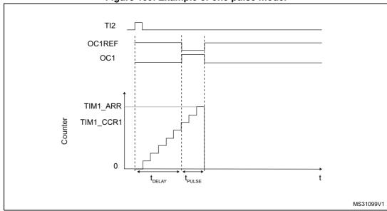
Figure 139. Example of one pulse mode.
