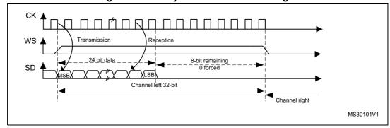
Figure 324. MSB justified 24-bit frame length
