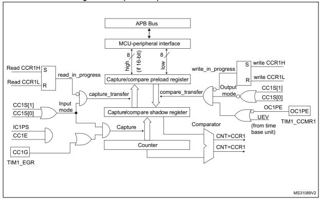
Figure 120. Capture/compare channel 1 main circuit
