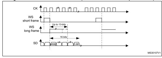
Figure 333. PCM standard waveforms (16-bit extended to 32-bit packet frame)
