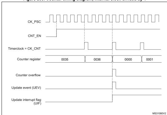
Figure 203. Counter timing diagram, internal clock divided by 4
