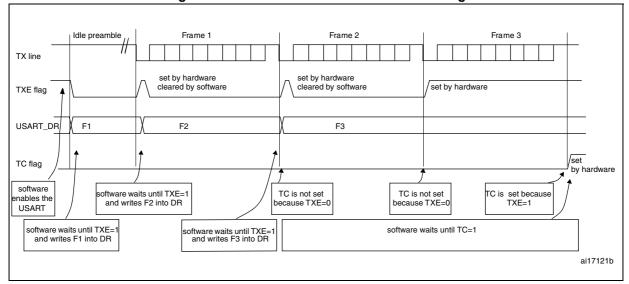
Figure 277. TC/TXE behavior when transmitting
