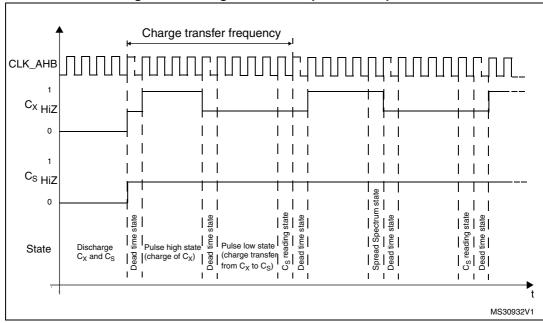
Figure 90. Charge transfer acquisition sequence
