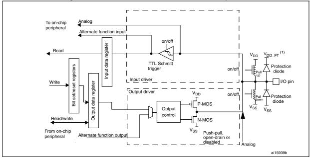
1.  $V_{DD\ FT}$  is a potential specific to five-volt tolerant I/Os and different from  $V_{DD}$ .
