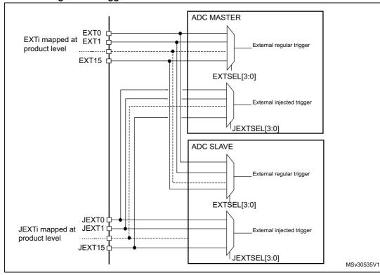
Figure 34. Triggers are shared between ADC master & ADC slave
