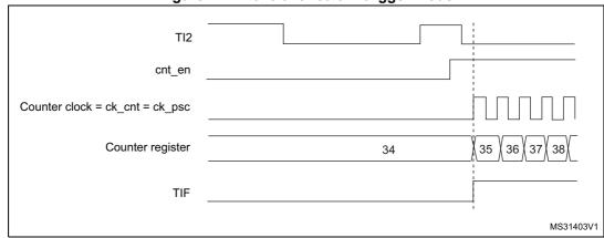
Figure 147. Control circuit in trigger mode
