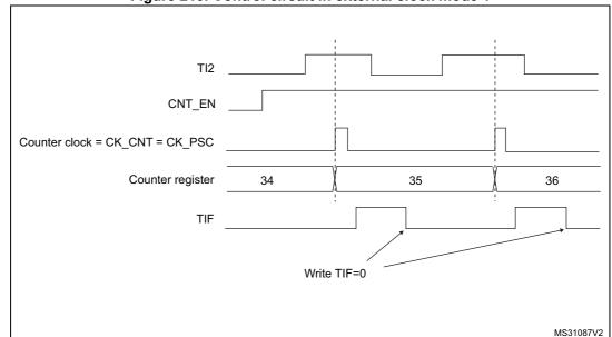
Figure 210. Control circuit in external clock mode 1
