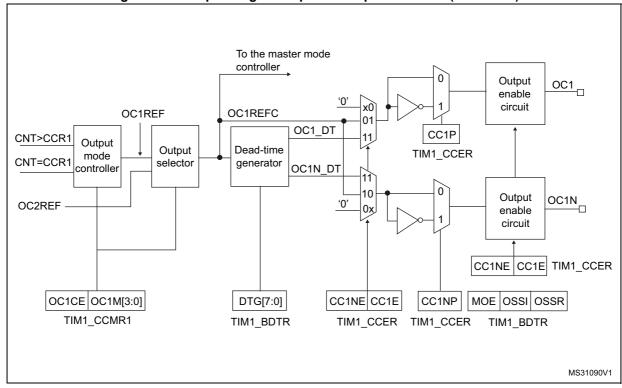
Figure 213. Output stage of capture/compare channel (channel 1)
