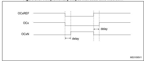
Figure 219. Complementary output with dead-time insertion.
