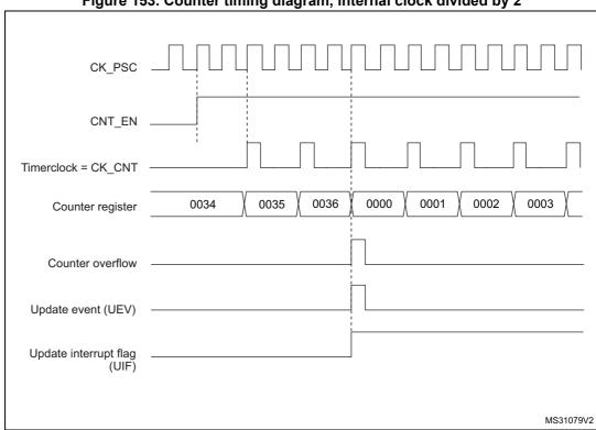
Figure 153. Counter timing diagram, internal clock divided by 2
