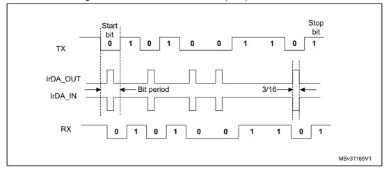
Figure 292. IrDA data modulation (3/16) -Normal Mode
