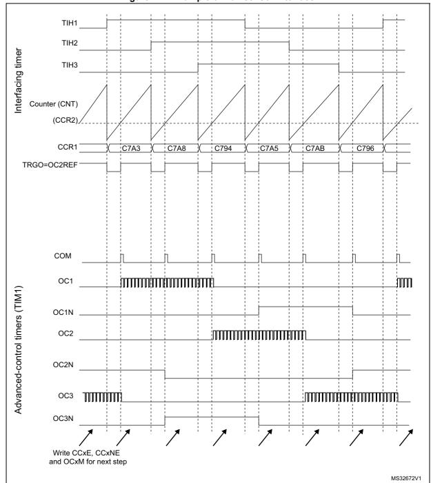
Figure 144. Example of Hall sensor interface
