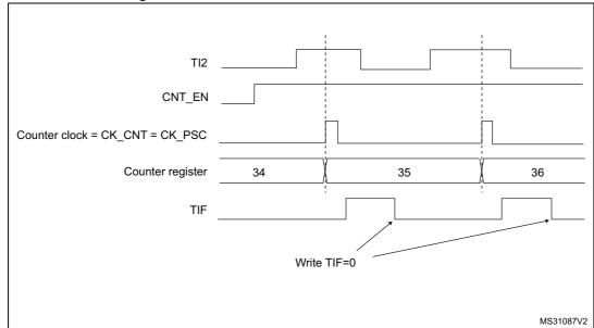
Figure 116. Control circuit in external clock mode 1
