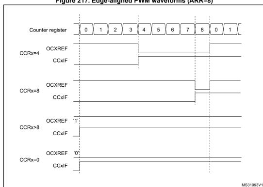
Figure 217. Edge-aligned PWM waveforms (ARR=8)
