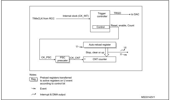
Figure 228. Basic timer block diagram
