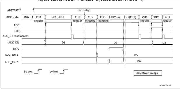
Figure 62. AUTODLY=1 in auto- injected mode (JAUTO=1)
