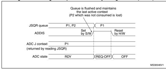
Figure 46. Flushing JSQR queue of context by setting ADDIS=1 (JQM=0)
