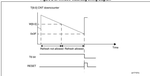
Figure 240. Window watchdog timing diagram
