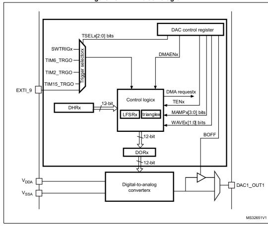
Figure 70. DAC1 block diagram
