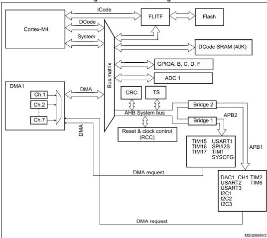
Figure 20. DMA block diagram
