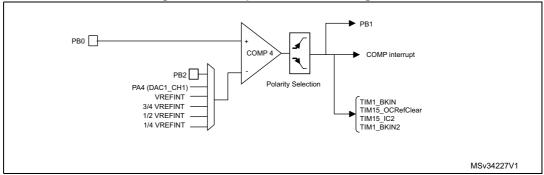
Figure 79. Comparator 6 block diagram
