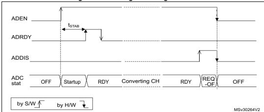
Figure 30. Enabling / Disabling the ADC
