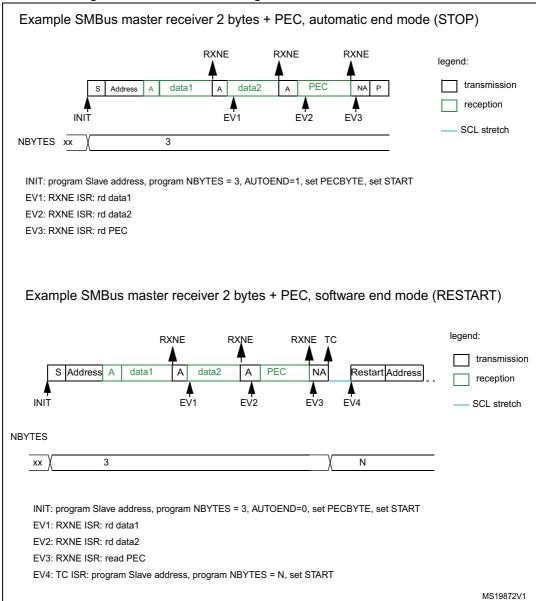
Figure 272. Bus transfer diagrams for SMBus master receiver
