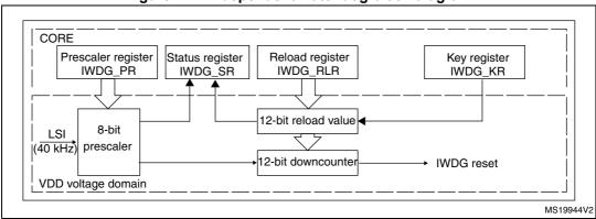
Figure 241. Independent watchdog block diagram
