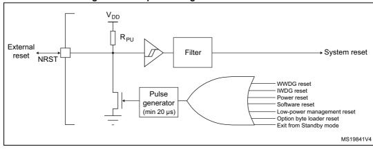
Figure 10. Simplified diagram of the reset circuit
