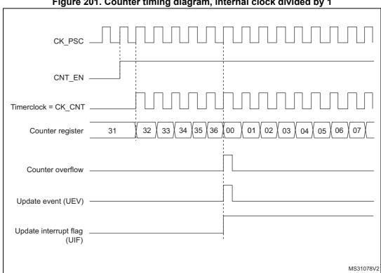
Figure 201. Counter timing diagram, internal clock divided by 1
