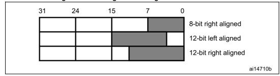
Figure 71. Data registers in single DAC channel mode
