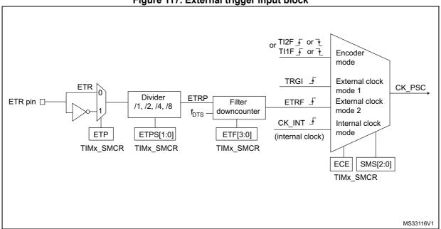
Figure 117. External trigger input block
