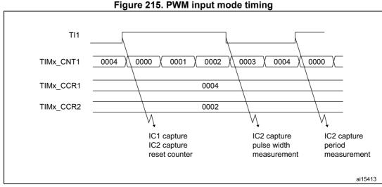
The PWM input mode can be used only with the TIMx\_CH1/TIMx\_CH2 signals due to the fact that only TI1FP1 and TI2FP2 are connected to the slave mode controller.
