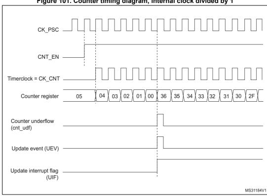
Figure 101. Counter timing diagram, internal clock divided by 1
