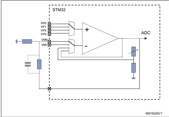
Figure 83. Standalone mode: external gain setting mode
