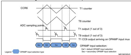
Figure 82. Timer controlled Multiplexer mode
