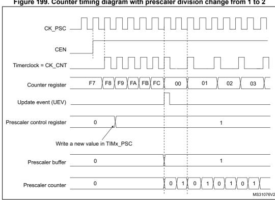
Figure 199. Counter timing diagram with prescaler division change from 1 to 2
