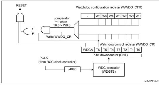
Figure 239. Watchdog block diagram
