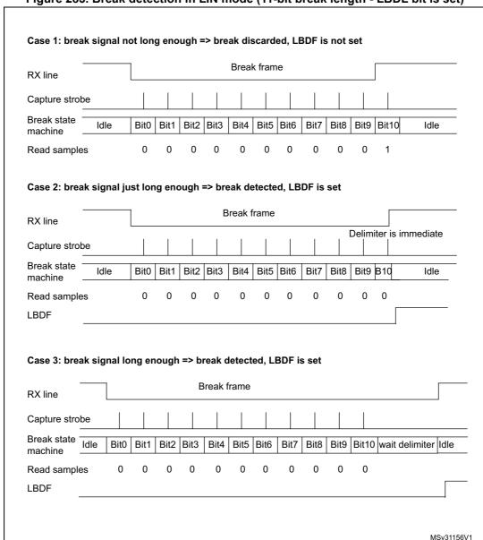
Figure 283. Break detection in LIN mode (11-bit break length - LBDL bit is set)
