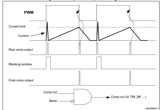
Figure 80. Comparator output blanking
