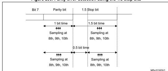
Figure 290. Parity error detection using the 1.5 stop bits
