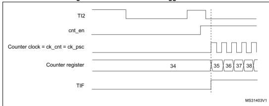
Figure 190. Control circuit in trigger mode
