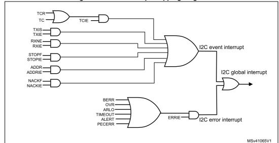
Figure 273. I2C interrupt mapping diagram
