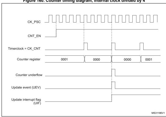
Figure 160. Counter timing diagram, internal clock divided by 4
