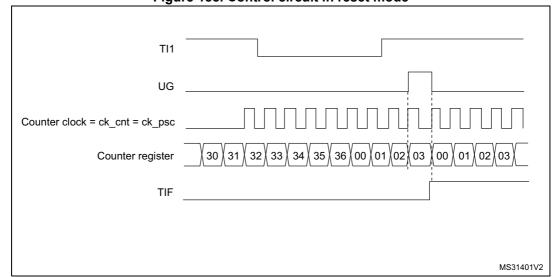
Figure 188. Control circuit in reset mode
