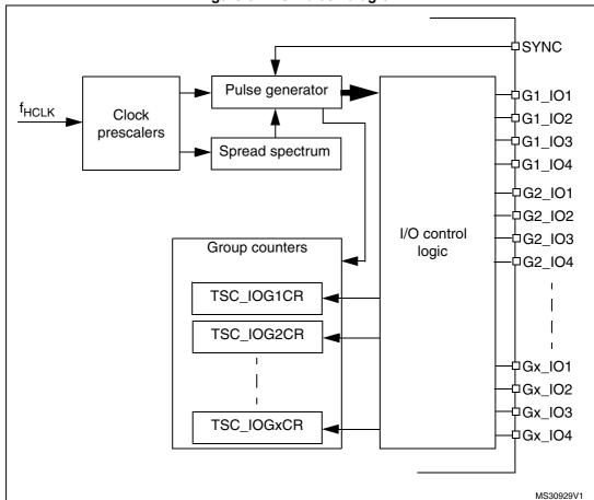
Figure 87. TSC block diagram
