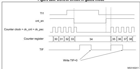
Figure 226. Control circuit in gated mode
