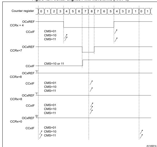
Figure 127. Center-aligned PWM waveforms (ARR=8)
