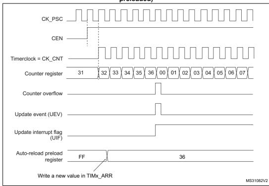
Figure 205. Counter timing diagram, update event when ARPE=0 (TIMx\_ARR not preloaded)
