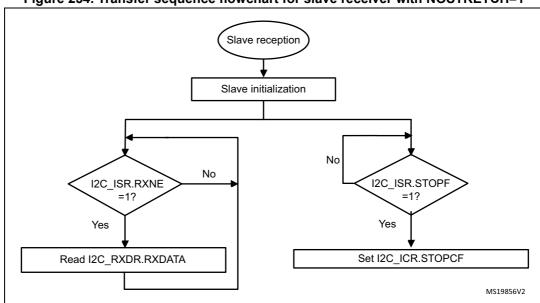
Figure 254. Transfer sequence flowchart for slave receiver with NOSTRETCH=1
