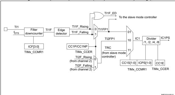
Figure 119. Capture/compare channel (example: channel 1 input stage)
