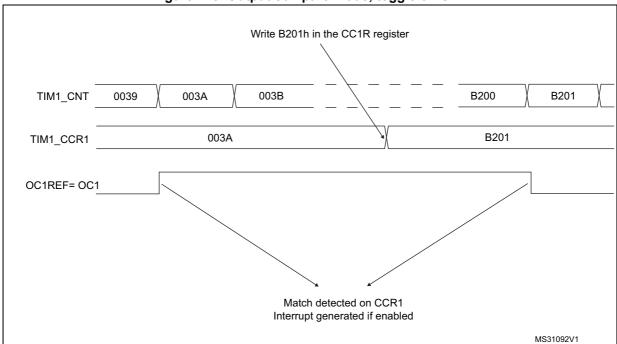
Figure 178. Output compare mode, toggle on OC1
