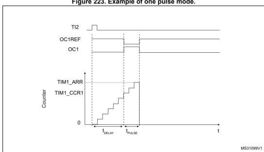
Figure 223. Example of one pulse mode.
