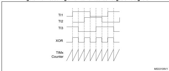
Figure 143. Measuring time interval between edges on 3 signals
