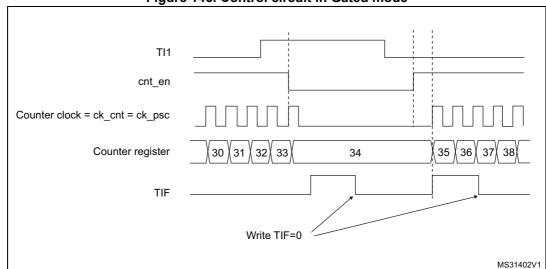
Figure 146. Control circuit in Gated mode
