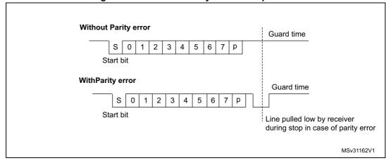
Figure 289. ISO 7816-3 asynchronous protocol
