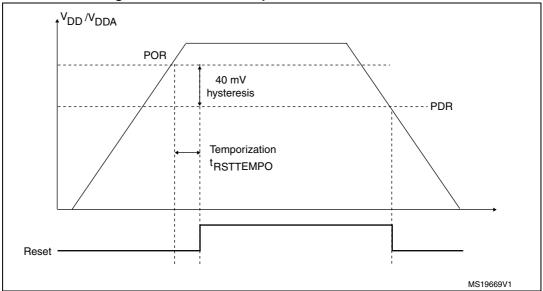
Figure 8. Power on reset/power down reset waveform
