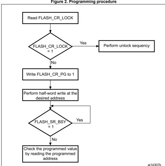
Figure 2. Programming procedure
