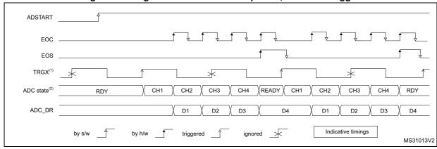
Figure 51. Single conversions of a sequence, hardware trigger
