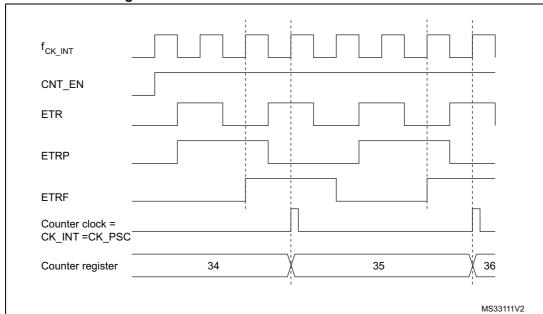
Figure 173. Control circuit in external clock mode 2
