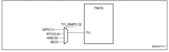
The input capture channel of the Timer 16 can be a GPIO line or an internal clock of the MCU. This selection is performed through the TI1\_RMP [1:0] bits in the TIM16\_OR register. The possibilities available are the following ones.
