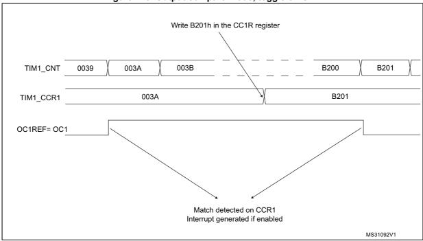
Figure 125. Output compare mode, toggle on OC1
