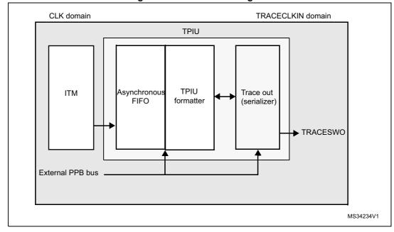
Figure 340. TPIU block diagram
