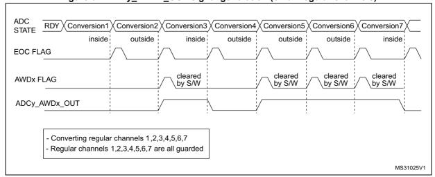
Figure 64. ADCy AWDx OUT signal generation (on all regular channels)
