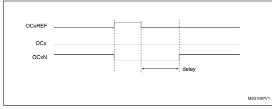
Figure 133. Dead-time waveforms with delay greater than the positive pulse
