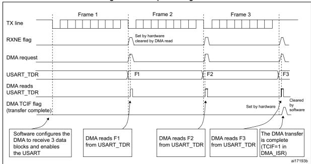
Figure 294. Reception using DMA
