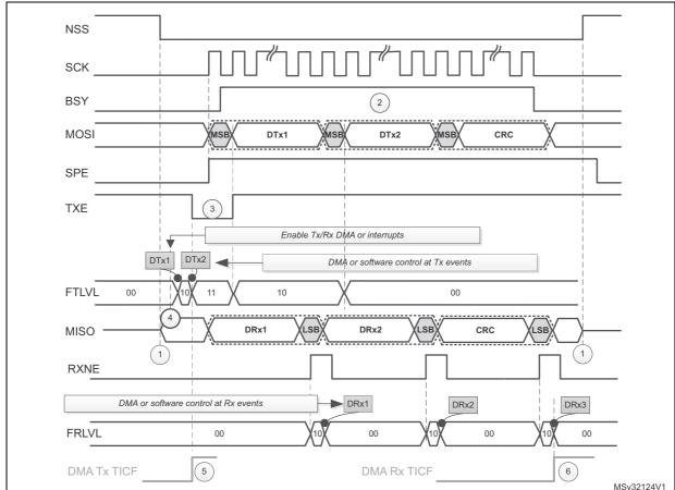
Figure 311. Master full duplex communication with CRC
