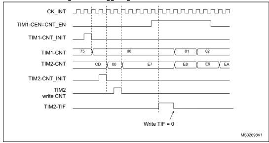
Figure 196. Triggering TIM2 with Enable of TIM1
