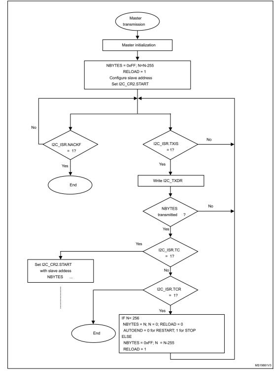
Figure 261. Transfer sequence flowchart for I2C master transmitter for N>255 bytes
