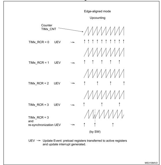
Figure 207. Update rate examples depending on mode and TIMx\_RCR register settings
