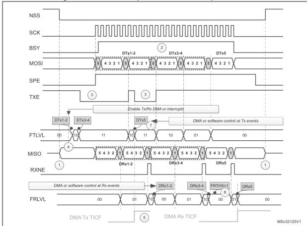
Figure 312. Master full duplex communication in packed mode
