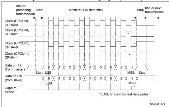
Figure 287. USART data clock timing diagram (M bits = 01)
