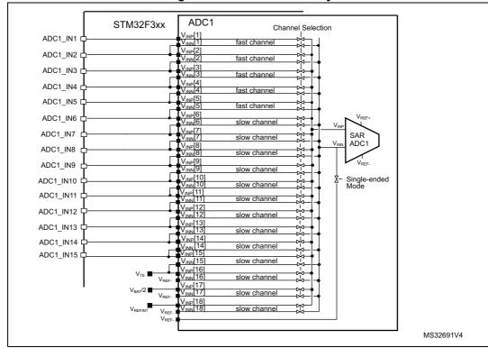
Figure 26. ADC1 connectivity
