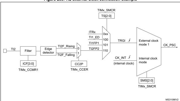
Figure 209. TI2 external clock connection example
