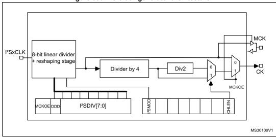
Figure 336. I<sup>2</sup>S clock generator architecture
