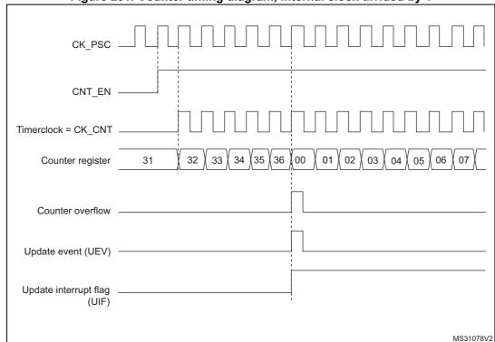
Figure 231. Counter timing diagram, internal clock divided by 1
