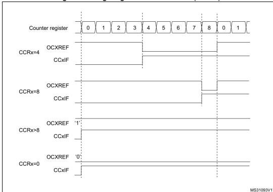
Figure 126. Edge-aligned PWM waveforms (ARR=8)
