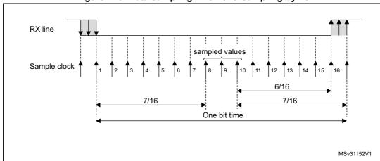
Figure 279. Data sampling when oversampling by 16
