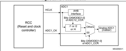
Figure 25. ADC clock scheme
