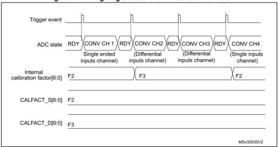
Figure 29. Mixing single-ended and differential channels
