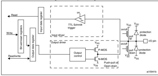
Figure 17. Output configuration
