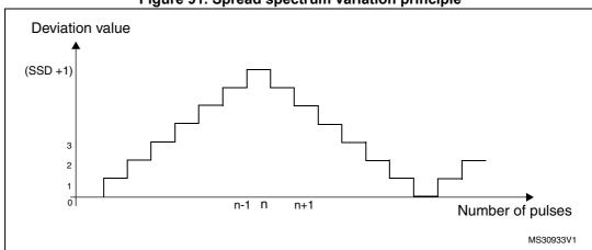
Figure 91. Spread spectrum variation principle
