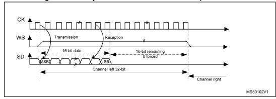
Figure 325. MSB justified 16-bit extended to 32-bit packet frame
