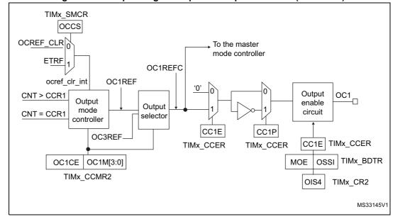
Figure 176. Output stage of capture/compare channel (channel 1)
