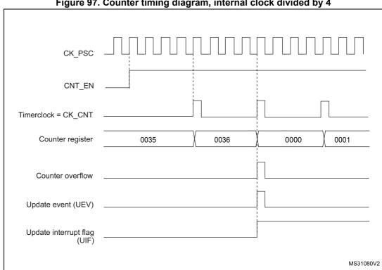
Figure 97. Counter timing diagram, internal clock divided by 4
