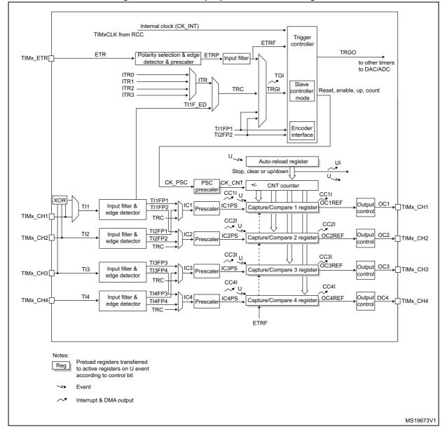
Figure 149. General-purpose timer block diagram
