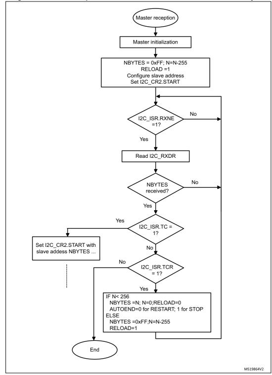
Figure 264. Transfer sequence flowchart for I2C master receiver for N >255 bytes
