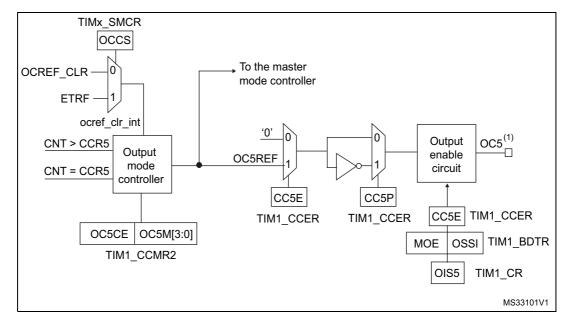
Figure 123. Output stage of capture/compare channel (channel 5, idem ch. 6)
