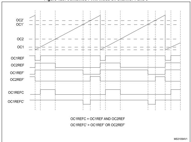
Figure 129. Combined PWM mode on channel 1 and 3
