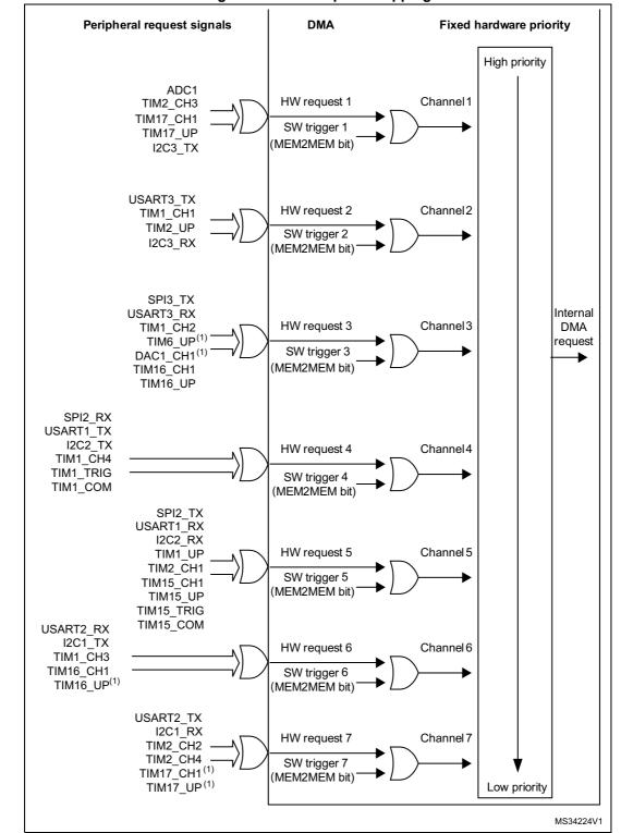
Figure 21. DMA request mapping
