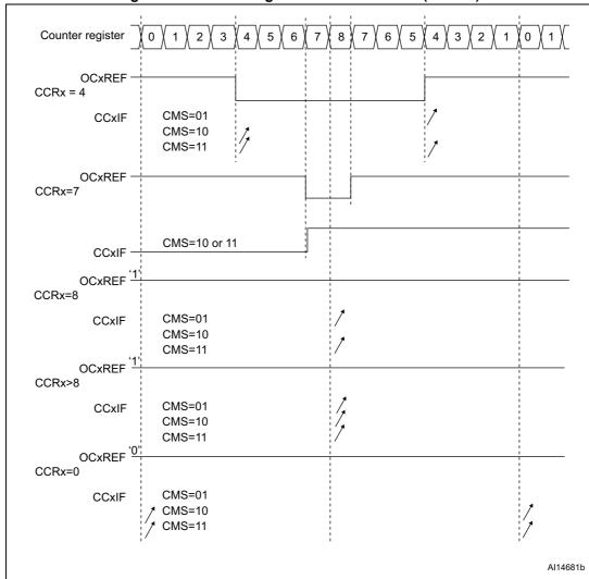
Figure 180. Center-aligned PWM waveforms (ARR=8)
