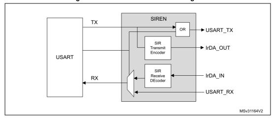
Figure 291. IrDA SIR ENDEC- block diagram
