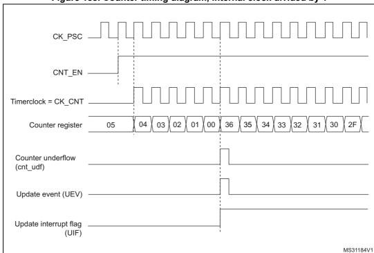
Figure 158. Counter timing diagram, internal clock divided by 1
