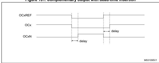
Figure 131. Complementary output with dead-time insertion
