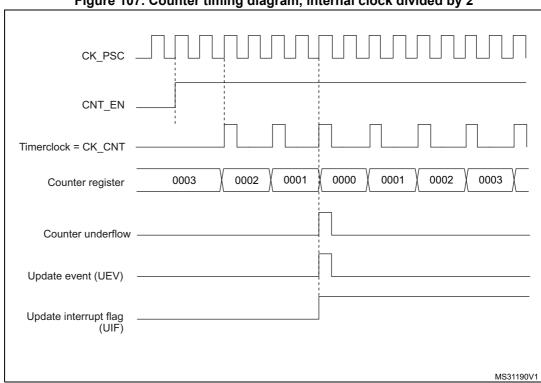
Figure 107. Counter timing diagram, internal clock divided by 2
