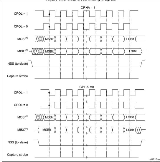
Figure 306. Data clock timing diagram
