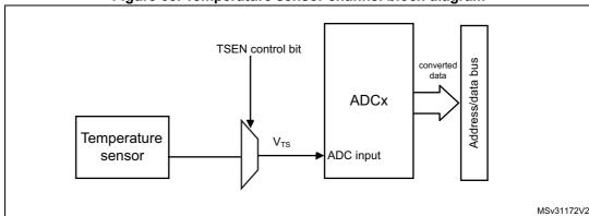
Figure 68. Temperature sensor channel block diagram
