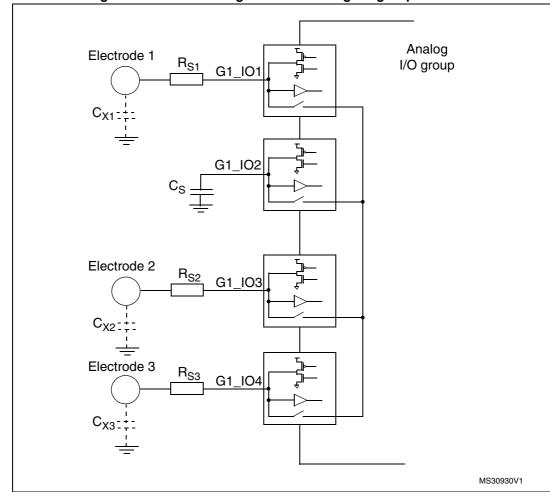
Figure 88. Surface charge transfer analog I/O group structure
