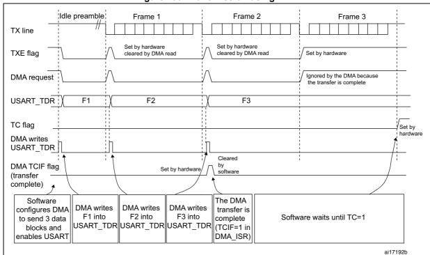
Figure 293. Transmission using DMA
