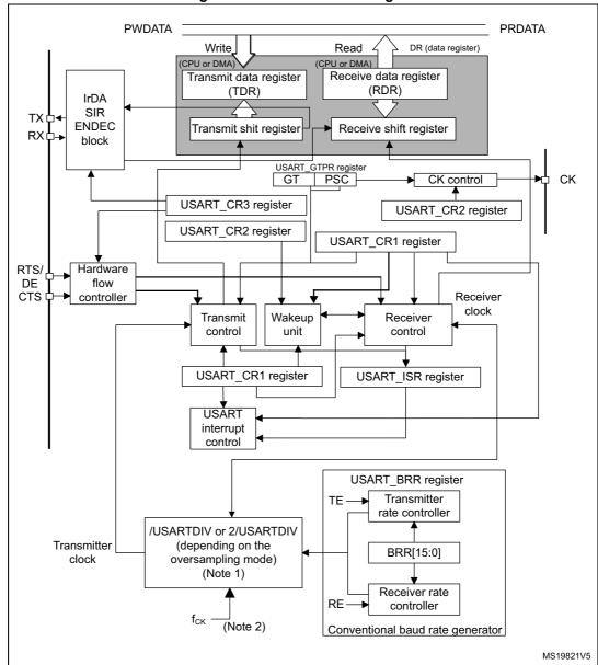
Figure 274. USART block diagram
