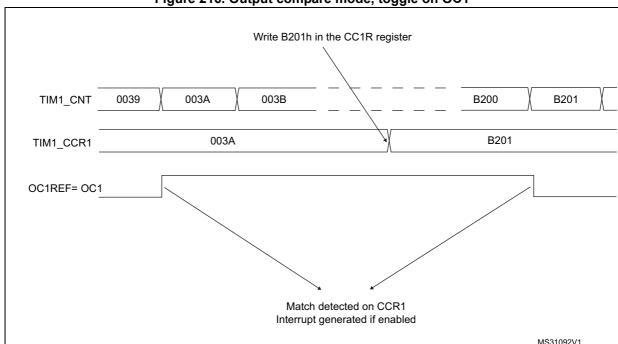
Figure 216. Output compare mode, toggle on OC1
