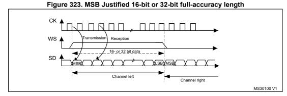
Data are latched on the falling edge of CK (for transmitter) and are read on the rising edge (for the receiver).
