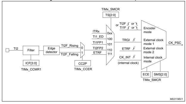
Figure 115. TI2 external clock connection example
