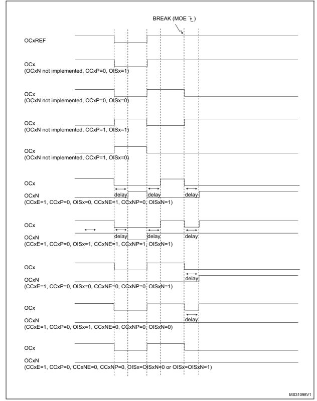
Figure 222. Output behavior in response to a break
