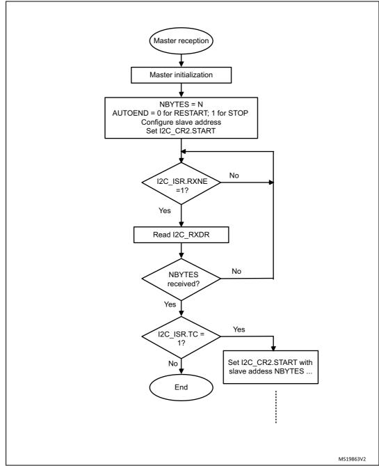
Figure 263. Transfer sequence flowchart for I2C master receiver for N≤255 bytes
