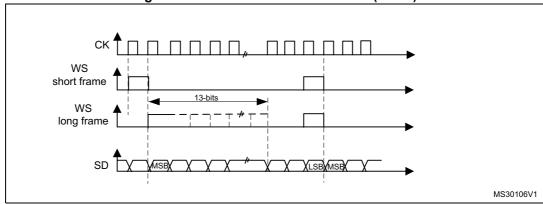
Figure 332. PCM standard waveforms (16-bit)
