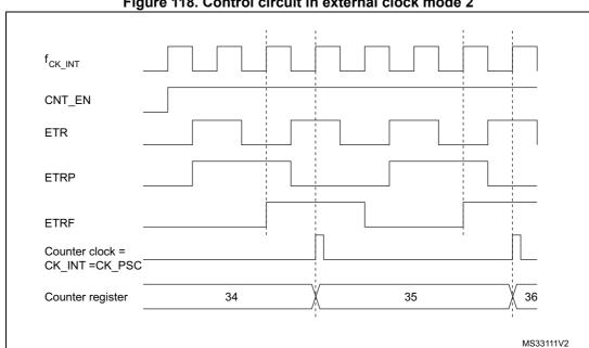
Figure 118. Control circuit in external clock mode 2
