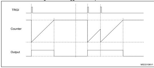
Figure 140. Retriggerable one pulse mode
