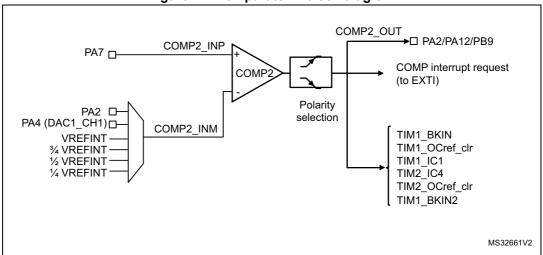
Figure 78. Comparator 4 block diagram
