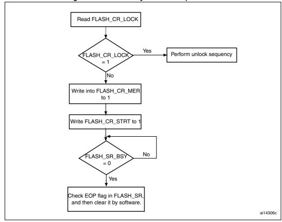
Figure 4. Flash memory Mass Erase procedure
