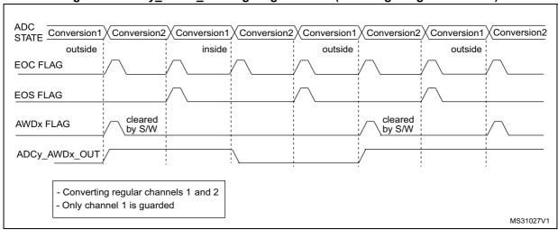
Figure 67. ADCy\_AWDx\_OUT signal generation (on all injected channels)
