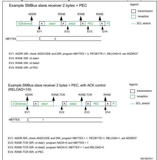
Figure 270. Bus transfer diagrams for SMBus slave receiver (SBC=1)
