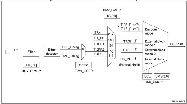
Figure 170. TI2 external clock connection example
