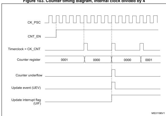
Figure 103. Counter timing diagram, internal clock divided by 4
