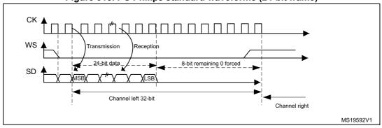
Figure 318. I<sup>2</sup>S Philips standard waveforms (24-bit frame)
