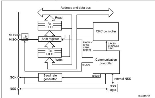
Figure 299. SPI block diagram
