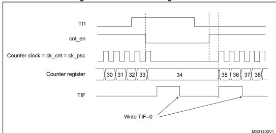
Figure 189. Control circuit in gated mode
