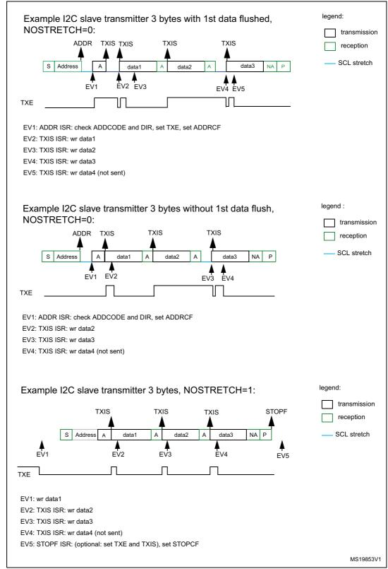
Figure 252. Transfer bus diagrams for I2C slave transmitter
