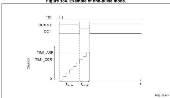
Figure 184. Example of one-pulse mode.
