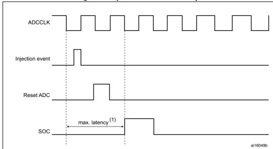
Figure 35. Injected conversion latency
