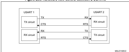
Figure 295. Hardware flow control between 2 USARTs
