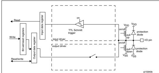
Figure 16. Input floating/pull up/pull down configurations
