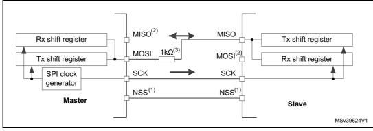
Figure 301. Half-duplex single master/ single slave application
