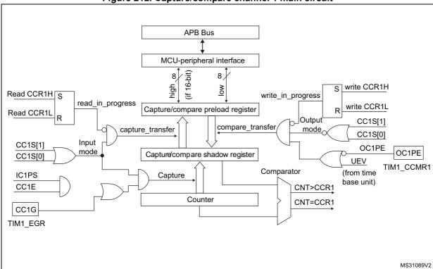
Figure 212. Capture/compare channel 1 main circuit
