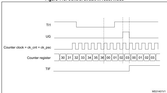
Figure 145. Control circuit in reset mode
