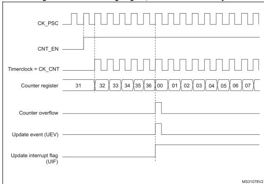
Figure 152. Counter timing diagram, internal clock divided by 1
