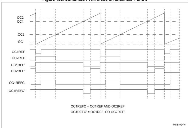
Figure 182. Combined PWM mode on channels 1 and 3
