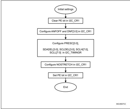
Figure 246. I2C initialization flowchart
