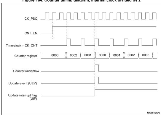
Figure 164. Counter timing diagram, internal clock divided by 2
