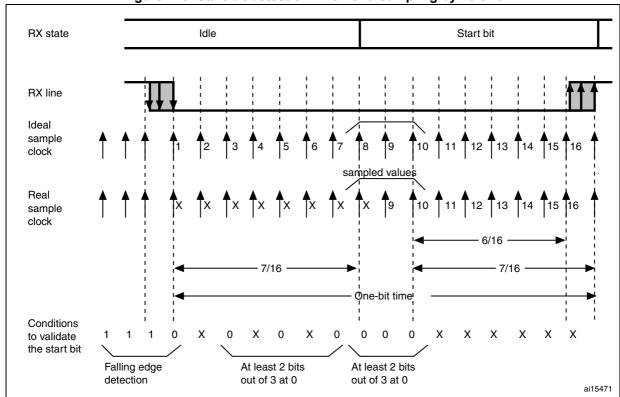
Figure 278. Start bit detection when oversampling by 16 or 8
