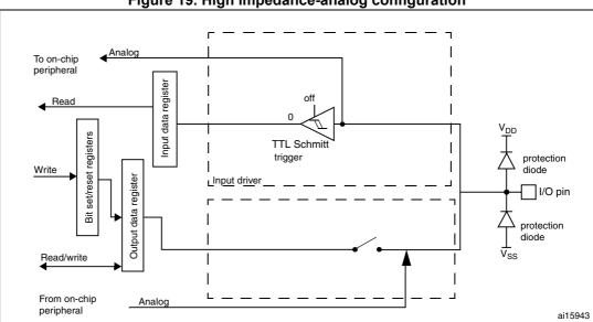
Figure 19. High impedance-analog configuration
