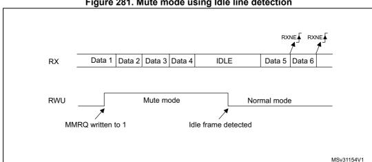
Figure 281. Mute mode using Idle line detection
