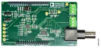
Figure 9. EVAL-CN0398-ARDZ Shield Board
