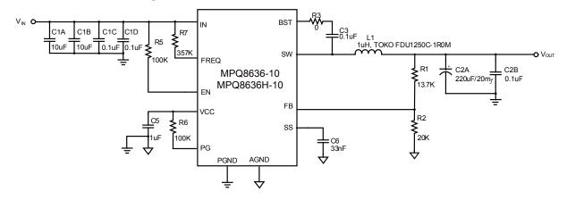
Figure 10 — Typical Application Circuit with No External Ramp MPQ8636-10, MPQ8636H-10,  $V_{IN}$ =12V,  $V_{OUT}$ =1V,  $I_{OUT}$ =10A,  $f_{SW}$ =500kHz
