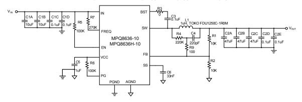
Figure 26 — Typical Application Circuit with Low ESR Ceramic Capacitor MPQ8636-10, MPQ8636H-10, V<sub>IN</sub>=12V, V<sub>OUT</sub>=1.2V, I<sub>OUT</sub>=10A, f<sub>SW</sub>=800kHz
