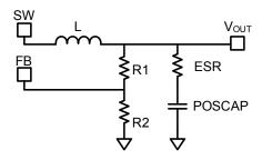
Figure 7—Simplified POSCAP Circuit
