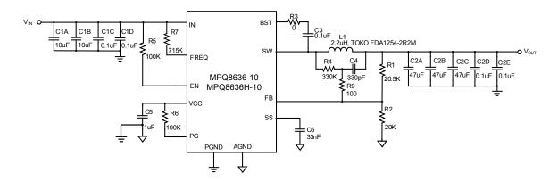
Figure 22 — Typical Application Circuit with Low ESR Ceramic Capacitor MPQ8636-10, MPQ8636H-10, V<sub>IN</sub>=12V, V<sub>OUT</sub>=1.2V, I<sub>OUT</sub>=10A, f<sub>SW</sub>=300kHz
