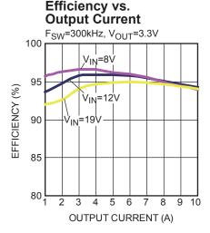
Figure 41 — Efficiency Curve MPQ8636-10, MPQ8636H-10,  $V_{OUT}$ =3.3V,  $I_{OUT}$ =1A-10A,  $f_{SW}$ =300kHz
