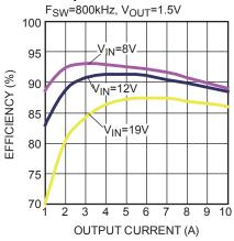
Figure 33 — Efficiency Curve MPQ8636-10, MPQ8636H-10,  $V_{OUT}$ =1.5V,  $I_{OUT}$ =1A-10A,  $f_{SW}$ =800kHz
