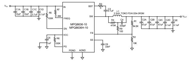
Figure 48 — Typical Application Circuit with Low ESR Ceramic Capacitor MPQ8636-10, MPQ8636H-10, V<sub>IN</sub>=12V, V<sub>OUT</sub>=5 V, I<sub>OUT</sub>=10A, f<sub>SW</sub>=500kHz
