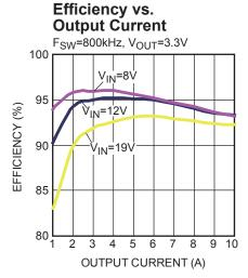
Figure 45 — Efficiency Curve MPQ8636-10, MPQ8636H-10,  $V_{OUT}$ =3.3V,  $I_{OUT}$ =1A-10A,  $f_{SW}$ =800kHz
