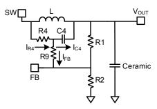
Figure 5—Simplified Circuit in PWM Mode with External Ramp Compensation
