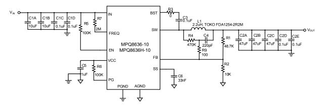
Figure 40 — Typical Application Circuit with Low ESR Ceramic Capacitor MPQ8636-10, MPQ8636H-10, V<sub>IN</sub>=12V, V<sub>OUT</sub>=3.3 V, I<sub>OUT</sub>=10A, f<sub>SW</sub>=300kHz
