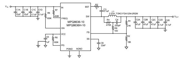
Figure 38 — Typical Application Circuit with Low ESR Ceramic Capacitor MPQ8636-10, MPQ8636H-10, V<sub>IN</sub>=12V, V<sub>OUT</sub>=1.8 V, I<sub>OUT</sub>=10A, f<sub>SW</sub>=800kHz
