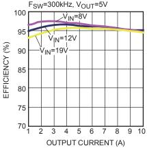
Figure 47 — Efficiency Curve MPQ8636-10, MPQ8636H-10, V<sub>OUT</sub>=5V, I<sub>OUT</sub>=1A-10A, f<sub>SW</sub>=300kHz
