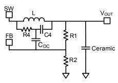
Figure 9—Simplified Ceramic Capacitor Circuit with DC-Blocking Capacitor
