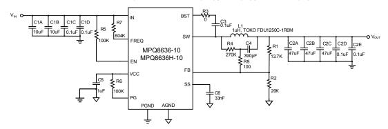
Figure 14 — Typical Application Circuit with Low ESR Ceramic Capacitor MPQ8636-10, MPQ8636H-10, V<sub>IN</sub>=12V, V<sub>OUT</sub>=1V, I<sub>OUT</sub>=10A, f<sub>SW</sub>=300kHz
