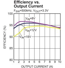
Figure 43 — Efficiency Curve
