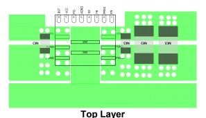
Figure 53—Recommend Input Capacitor
