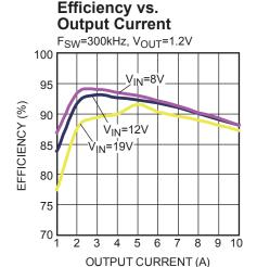
$\label{eq:figure 23} \textbf{Figure 23} \leftarrow \textbf{Efficiency Curve} \\ \textbf{MPQ8636-10, MPQ8636H-10, } \textbf{V}_{\text{OUT}} = \textbf{1.2V, } \textbf{I}_{\text{OUT}} = \textbf{1A-10A, } \textbf{f}_{\text{SW}} = \textbf{300kHz} \\ \\ \textbf{MPQ8636-10, MPQ8636H-10, } \textbf{V}_{\text{OUT}} = \textbf{1.2V, } \textbf{I}_{\text{OUT}} = \textbf{1.2V, }$
