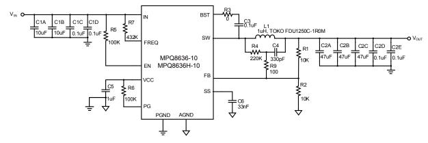
Figure 24 — Typical Application Circuit with Low ESR Ceramic Capacitor MPQ8636-10, MPQ8636H-10, V<sub>IN</sub>=12V, V<sub>OUT</sub>=1.2V, I<sub>OUT</sub>=10A, f<sub>SW</sub>=500kHz
