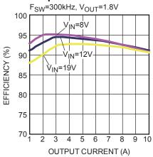
Figure 35 — Efficiency Curve MPQ8636-10, MPQ8636H-10,  $V_{OUT}$ =1.8V,  $I_{OUT}$ =1A-10A,  $f_{SW}$ =300kHz
