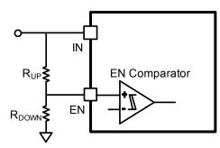
Figure 6—Adjustable UVLO Threshold
