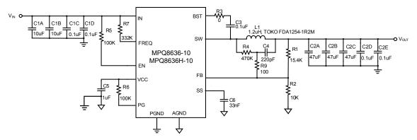
Figure 32 — Typical Application Circuit with Low ESR Ceramic Capacitor MPQ8636-10, MPQ8636H-10, V<sub>IN</sub>=12V, V<sub>OUT</sub>=1.5 V, I<sub>OUT</sub>=10A, f<sub>SW</sub>=800kHz
