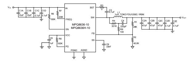
Figure 16 — Typical Application Circuit with Low ESR Ceramic Capacitor MPQ8636-10, MPQ8636H-10, V<sub>IN</sub>=12V, V<sub>OUT</sub>=1V, I<sub>OUT</sub>=10A, f<sub>SW</sub>=800kHz
