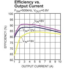
Figure 21 — Efficiency Curve MPQ8636-10, MPQ8636H-10,  $V_{OUT}$ =0.8V,  $I_{OUT}$ =1A-10A,  $f_{SW}$ =500kHz
