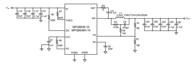
Figure 28 — Typical Application Circuit with Low ESR Ceramic Capacitor MPQ8636-10, MPQ8636H-10, V<sub>IN</sub>=12V, V<sub>OUT</sub>=1.5 V, I<sub>OUT</sub>=10A, f<sub>SW</sub>=300kHz
