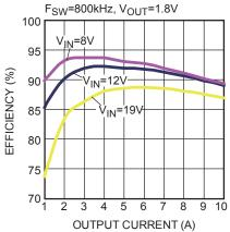
Figure 39 — Efficiency Curve MPQ8636-10, MPQ8636H-10, V<sub>OUT</sub>=1.8V, I<sub>OUT</sub>=1A-10A, f<sub>sw</sub>=800kHz
