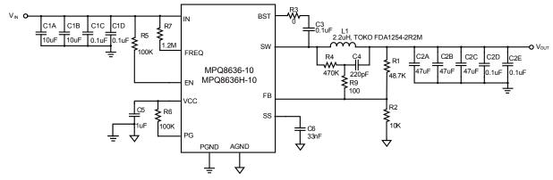
Figure 42 — Typical Application Circuit with Low ESR Ceramic Capacitor MPQ8636-10, MPQ8636H-10,  $V_{IN}$ =12V,  $V_{OUT}$ =3.3 V,  $I_{OUT}$ =10A,  $f_{SW}$ =500kHz
