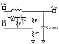
Figure 8—Simplified Ceramic Capacitor Circuit
