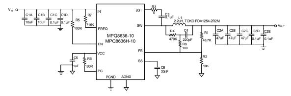
Figure 44 — Typical Application Circuit with Low ESR Ceramic Capacitor MPQ8636-10, MPQ8636H-10, V<sub>IN</sub>=12V, V<sub>OUT</sub>=3.3 V, I<sub>OUT</sub>=10A, f<sub>SW</sub>=800kHz
