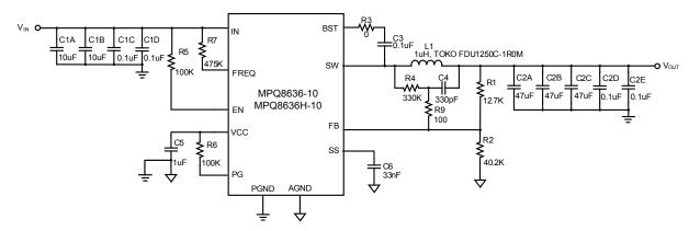
Figure 18 — Typical Application Circuit with Low ESR Ceramic Capacitor MPQ8636-10, MPQ8636H-10, V<sub>IN</sub>=12V, V<sub>OUT</sub>=0.8V, I<sub>OUT</sub>=10A, f<sub>SW</sub>=300kHz
