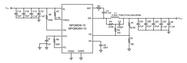
Figure 46 — Typical Application Circuit with Low ESR Ceramic Capacitor MPQ8636-10, MPQ8636H-10, V<sub>IN</sub>=12V, V<sub>OUT</sub>=5 V, I<sub>OUT</sub>=10A, f<sub>SW</sub>=300kHz
