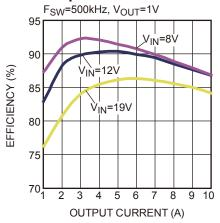
Figure 13 — Efficiency Curve MPQ8636-10, MPQ8636H-10, V<sub>OUT</sub>=1V, I<sub>OUT</sub>=1A-10A, f<sub>SW</sub>=500kHz
