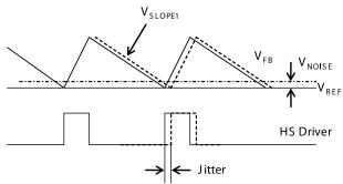
Figure 3—Jitter in PWM Mode
