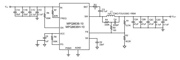
Figure 20 — Typical Application Circuit with Low ESR Ceramic Capacitor MPQ8636-10, MPQ8636H-10, V<sub>IN</sub>=12V, V<sub>OUT</sub>=0.8V, I<sub>OUT</sub>=10A, f<sub>SW</sub>=500kHz
