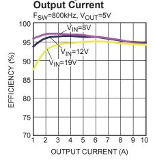
Figure 51 — Efficiency Curve MPQ8636-10, MPQ8636H-10,  $V_{OUT}$ =5V,  $I_{OUT}$ =1A-10A,  $f_{SW}$ =800kHz
