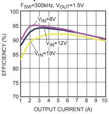
Figure 29 — Efficiency Curve
