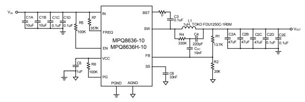
Figure 12 — Typical Application Circuit with Low ESR Ceramic Capacitor and DC-Blocking Capacitor.
