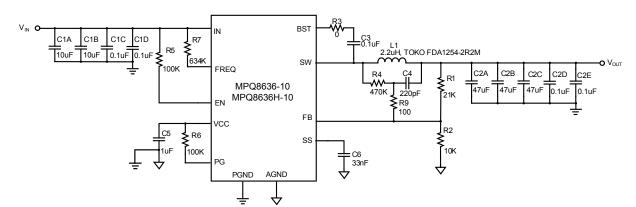
Figure 36 — Typical Application Circuit with Low ESR Ceramic Capacitor MPQ8636-10, MPQ8636H-10, V<sub>IN</sub>=12V, V<sub>OUT</sub>=1.8 V, I<sub>OUT</sub>=10A, f<sub>SW</sub>=500kHz
