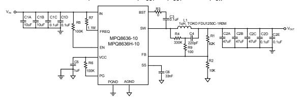
Figure 50 — Typical Application Circuit with Low ESR Ceramic Capacitor MPQ8636-10, MPQ8636H-10, V<sub>IN</sub>=12V, V<sub>OUT</sub>=5 V, I<sub>OUT</sub>=10A, f<sub>SW</sub>=800kHz Efficiency vs.
