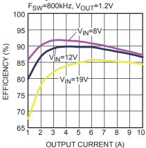
Figure 27 — Efficiency Curve MPQ8636-10, MPQ8636H-10,  $V_{OUT}$ =1.2V,  $I_{OUT}$ =1A-10A,  $f_{SW}$ =800kHz
