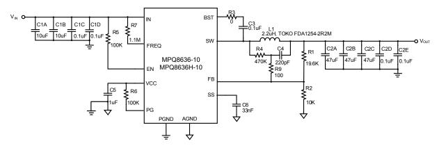
Figure 34 — Typical Application Circuit with Low ESR Ceramic Capacitor MPQ8636-10, MPQ8636H-10, V<sub>IN</sub>=12V, V<sub>OUT</sub>=1.8 V, I<sub>OUT</sub>=10A, f<sub>SW</sub>=300kHz
