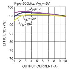
Figure 49 — Efficiency Curve MPQ8636-10, MPQ8636H-10,  $V_{OUT}$ =5V,  $I_{OUT}$ =1A-10A,  $f_{SW}$ =500kHz
