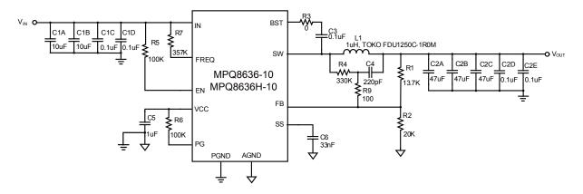
Figure 11 — Typical Application Circuit with Low ESR Ceramic Capacitor MPQ8636-10, MPQ8636H-10, V<sub>IN</sub>=12V, V<sub>OUT</sub>=1V, I<sub>OUT</sub>=10A, f<sub>SW</sub>=500kHz
