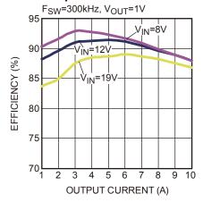
Figure 15 — Efficiency Curve MPQ8636-10, MPQ8636H-10, V<sub>OUT</sub>=1V, I<sub>OUT</sub>=1A-10A, f<sub>SW</sub>=300kHz
