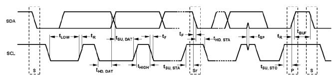
S = START CONDITION Sr = REPEATED START CONDITION P = STOP CONDITION
