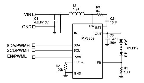
Figure 2: Typical Application for Single String 8LEDs
