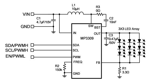
Figure 3: Typical Application for 3X3 LED Array
