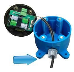
Plug the included wire harness into the receptacle on the circuit board inside the node.
