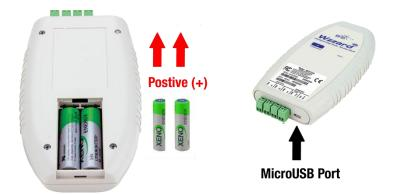
Remove back cover. Insert both batteries with the positive (+) towards the terminal blocks.
