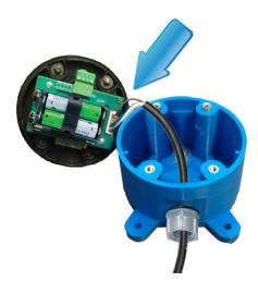
Connect your sensor to the wires running from the node's conduit. Consult the charts below for wire colors and connections.
