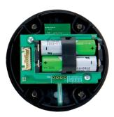
In most installations you will only need to place the batteries in the battery holder. But in high vibration environments you should also use the optional bettery retaining clip. Do not use excessive force while placing or removing the clip, as you can break it.
