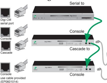
Connect Serial port on Digi CM to Console port on front of Digi RPM with RJ-45 cable provided (EP0601014).
