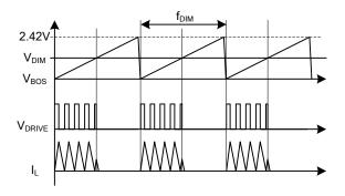
Figure 4: DC Burst Dimming
