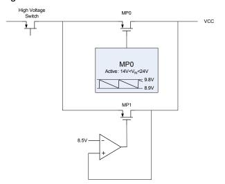
Figure 2: Functional Block Diagram of LDO
