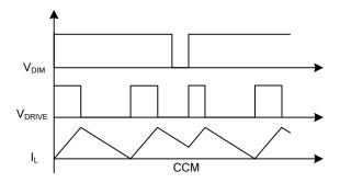
Figure 5: CCM in Large Dimming Duty
