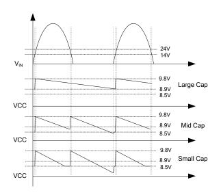
Figure 3: VCC Voltage in Different Capacitance
