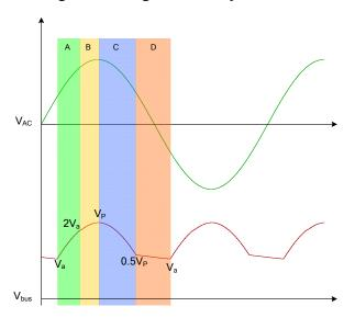
Figure 11: Waveform of Valley Fill Circuit
