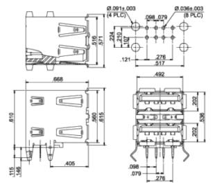
Description: USB Socket Type A Double Row Through Hole Plating Code: 30 Shell Plating: N/A
