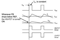
Figure 2: Heavy-Load Operation
