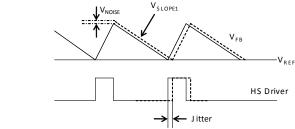
Figure 5: Jitter in PWM Mode
