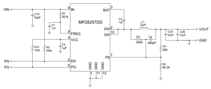
Figure 10: Typical Application Circuit V<sub>IN</sub>=12V, V<sub>OUT</sub>=1.2V, I<sub>OUT</sub>=4A
