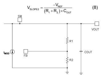
Figure 9: Simplified Circuit in Skip Mode
