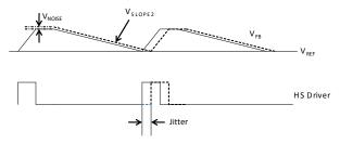
Figure 6: Jitter in Skip Mode
